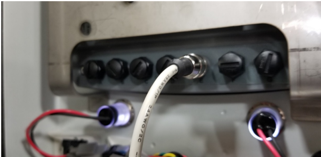
PROGRAMMING CABLE CONNECTED TO PORT E
