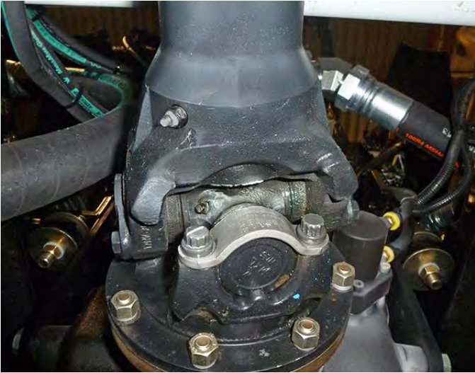
Drive Shaft Slip Yolk And U-joint Grease Points.
